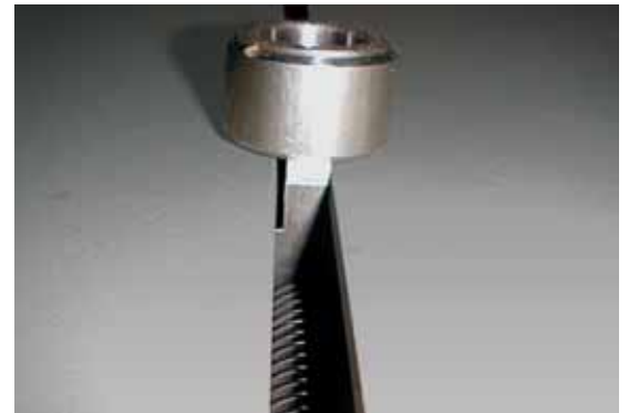
AutoSet C4 steel puck direct driven by servo-motor.
