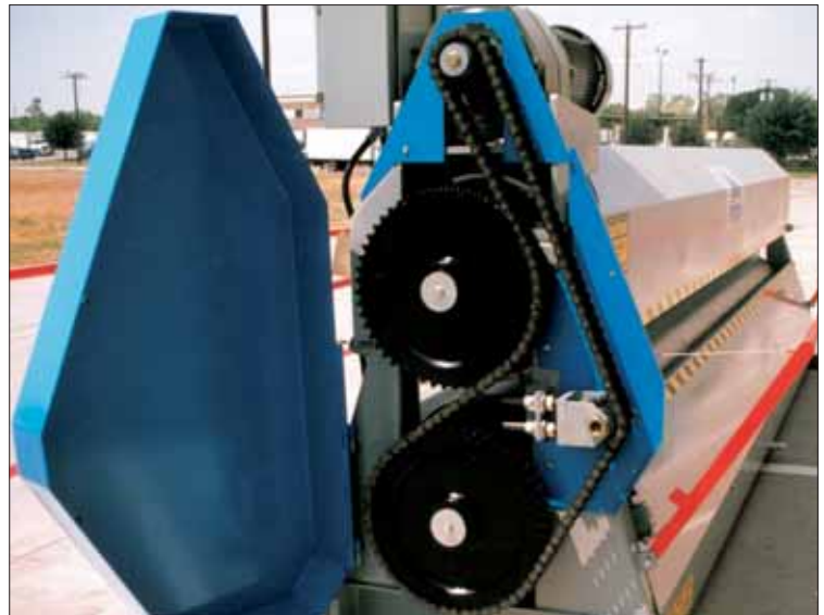
Right end with cover open. Extra heavy double-100 chain and rugged chain tensioner.
