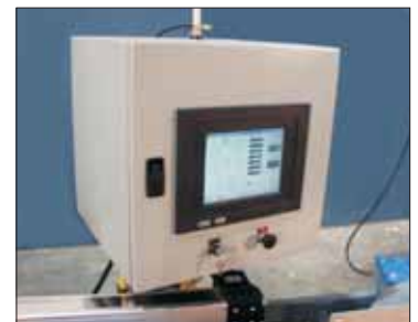
Operator interface with the computer control is a simple to use touchscreen panel.
